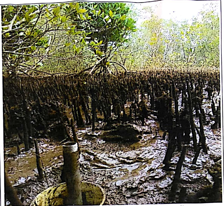
A plastic pipe is used to clear the top 30cms of sediment. The rods are then driven into the sediment until refusal. In the mangroves at Nahoon, most benchmarks were driven down to 3m.
