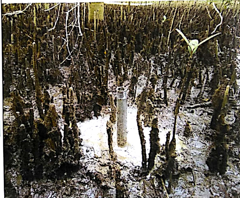
Receiving end of the benchmark which has been cemented in place. Measurements are taken by placing an arm-like instrument over this receiver. The instrument is rotated around the receiver and the height of the surrounding sediment is measured as a series of points. A profile of the sediment can then be generated.
