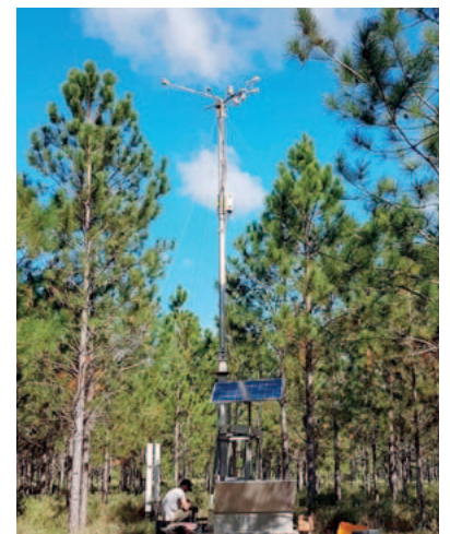
Mobile eddy covariance system measuring pine ET
