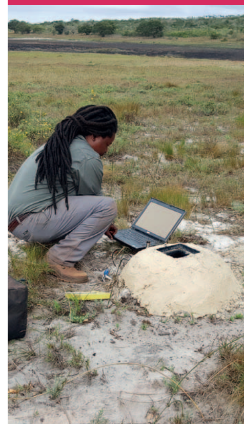
Mobile eddy covariance system measuring pine ET
